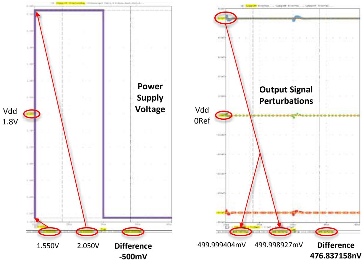
These waveforms illustrate an over-the-top amount of power disturbance. To go beyond any possible level of doubt, a 500mV 0.1ps Rise time step in power supply voltage was imposed – which created about 1 PPM (part-per-million) error in the output signal.
