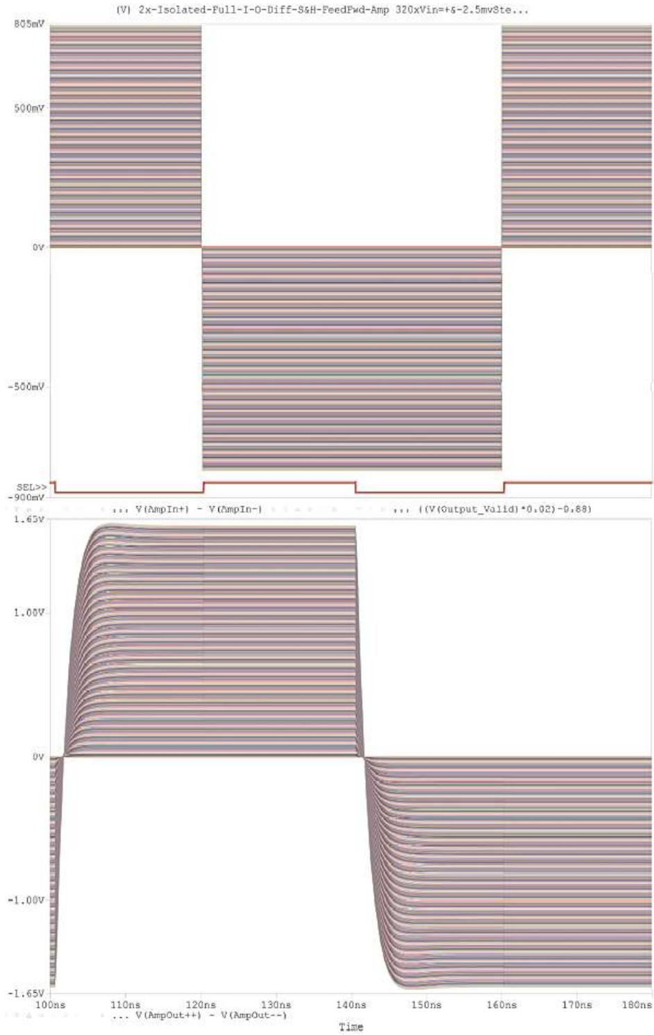
This is an example of 100% difference in adjacent component matching tolerance somewhere around the 2/3 level point. The error is undetectable to better than a PPM. No precision parts or trimmed components are required, facilitating precise divisions of the input voltage reference (64 steps of 20mV) as well as enabling other very precise analog operations without precision parts.
