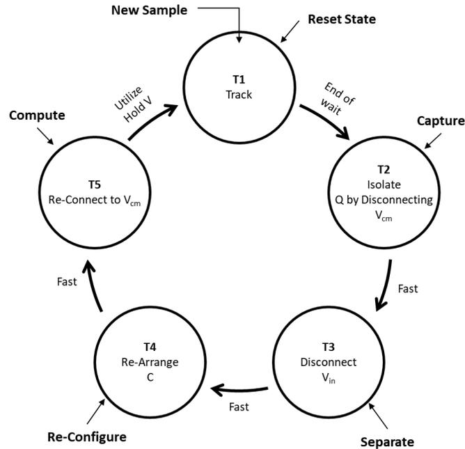
Figure 5 – Track & Hold state diagram
