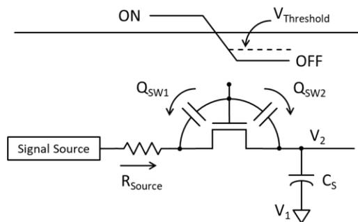
Figure 2.2 – MOSFET switch charge transfer capacitances at turnoff
