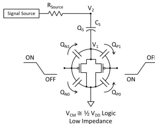
Figure 3.2 – Transmission-gate switch turnoff charge transfer capacitances
