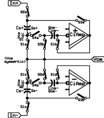
Figure 6.1 - 6.4 – State T1 = Track signal source voltage
