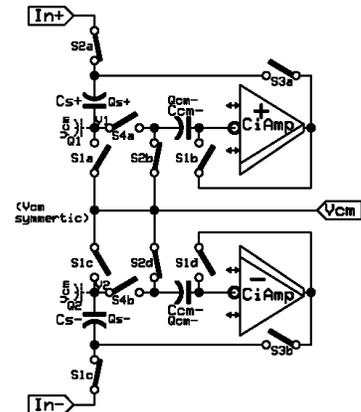
Figure 7.1 – 7.4 – State T2 = Isolate tracking capacitor(s) from analog ground ( $V_{cm}$ ) first
