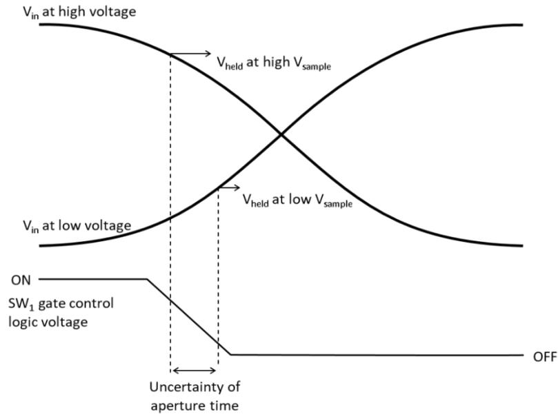
Figure 2.1 – Aperture time dependence on sampled signal voltage
